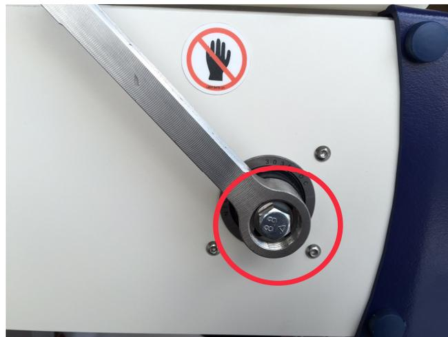
Figure 4 Tighten crank arm with 13mm socket wrench
