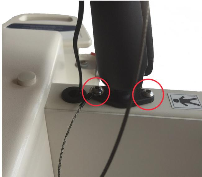
Figure 5 Bolts securing SAGE mounting
